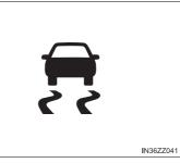
If the light stays on, the TCS, DSC or the brake assist system may have a malfunction and they may not operate correctly. Take your vehicle to your Scion dealer.
