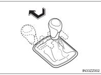
If shifting to R is difficult, shift back into neutral, release the clutch pedal, and try again.
