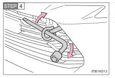
Tighten down the towing eyelet securely using a wheel nut wrench or hard metal bar.
