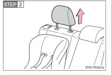
Secure the child restraint system using the seat belt or the LATCH anchors, and adjust the head restraint to the uppermost position.
