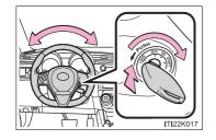
When starting the engine, the engine switch may seem stuck in the "LOCK" position. To free it, turn the key while turning the steering wheel slightly left and right.
