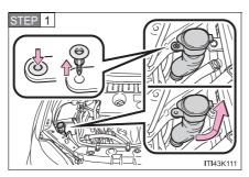
For easy access to the light bulbs, remove the securing clip and turn and pull off the washer fluid filler opener.
