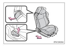
Lift the seatback lock release lever or seatback angle adjustment lever.
