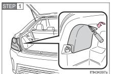
Open the back door and remove the cover.
