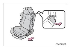
Lift the seatback lock release lever.
