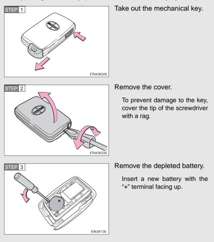
Replacing the battery (vehicles with a smart key system)
