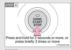
Vehicles with a smart key system: To stop the engine, press and hold the "ENGINE START STOP" switch for 2 consecutive seconds or more, or press it briefly 3 times or more in succession.
