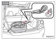
Hook the other end of the belt to the front cargo hook located diagonally to the used rear hook.
