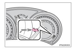
Items displayed can be switched by pressing the odometer/trip meter display change button.
