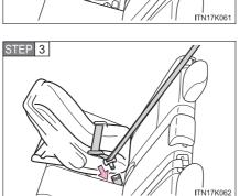
Run the seat belt through the child restraint system and insert the plate into the buckle. Make sure that the belt is not twisted.
