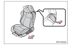
Lift the seatback lock release lever.
