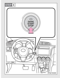
Press the "ENGINE START STOP" switch.
