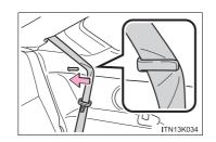
Pass the outboard seat belts through the seat belt hangers.
