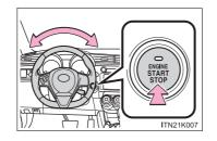
The green indicator light on the "ENGINE START STOP" switch will flash. Press the "ENGINE START STOP" switch again while turning the steering wheel left and right.
