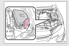
Under the driver's side instrument panel
