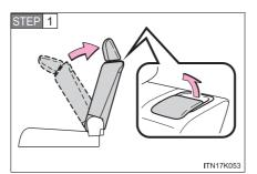
Fold the seatback while pulling the seatback angle adjustment lever up. Return the seatback and secure it at the first lock position.
