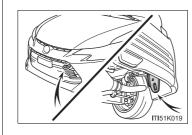
To help enhance safety, install the towing eyelet into the front left hole.
