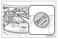
If the oil level is below or near the low level mark, add engine oil of the same type as that already in the engine.
