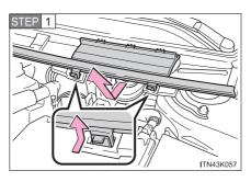
Disconnect the claws to remove the service cover as shown in the illustration.
