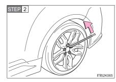
Slightly loosen the wheel nuts (one turn).
