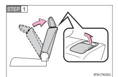
Fold the seatback while pulling the seatback angle adjustment lever up. Return the seatback and secure it at the first lock position.
