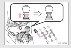
Shift the shift lever to R while lifting up the ring section.
