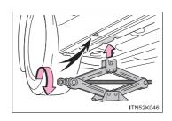
The jack point guides are located under the rocker panel. They indicate the jack point positions.
