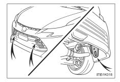
If a tow truck is not available in an emergency, your vehicle may be temporarily towed using a cable or chain secured to the emergency towing eyelets. This should only be attempted on hard surfaced roads for at most 50 miles (80 km) at under 18 mph (30 km/h).
