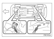
If your vehicle is transported by a flatbed truck, it should be tied down at the locations shown in the illustration.
