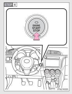
Press the "ENGINE START STOP" switch.
