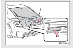
Raise the back door while pushing up the back door opener switch. Before driving
