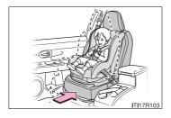
Only put a forward-facing child restraint system on the front seat when unavoidable. When installing a forward-facing child restraint system on the front passenger seat, move the seat as far back as possible even if the "AIR BAG OFF" indicator light is illuminated. Failure to do so may result in death or serious injury if the airbags deploy (inflate).
