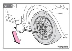
Slightly loosen the wheel nuts (one turn).
