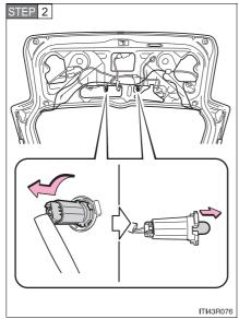
Open the back door and remove the trim board.
