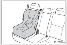
Seat belts equipped with a child restraint locking mechanism (ALR/ELR belts except driver's seat belt) ( $\rightarrow$ P. 47)
