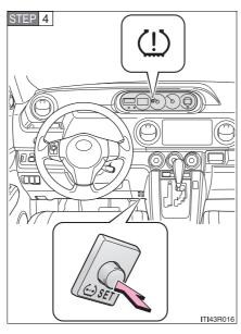
Press and hold the tire pressure warning reset button until the tire pressure warning light blinks slowly 3 times.
