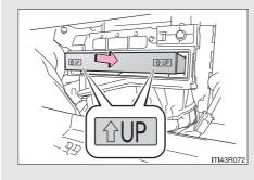
Replace the air conditioning filter with a new one.
