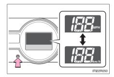
When the odometer is displayed, press and hold the odometer/trip meter and trip meter reset button to switch the display between MPH and km/h.
