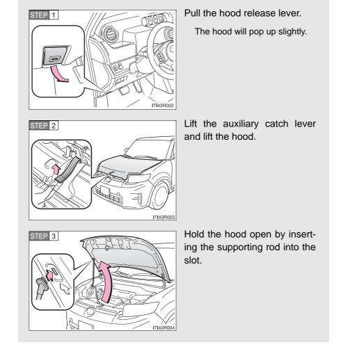
Release the lock from the inside of the vehicle to open the hood.
