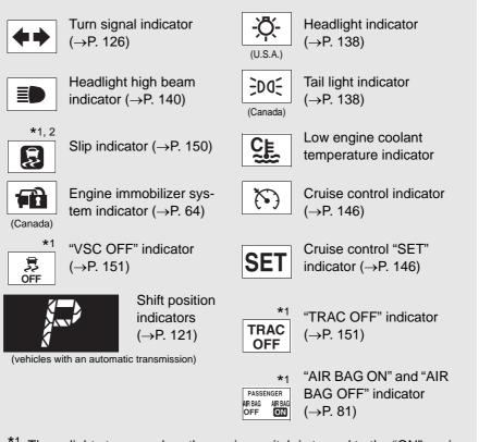
\*1: These lights turn on when the engine switch is turned to the "ON" position to indicate that a system check is being performed. They will turn off after the engine is started, or after a few seconds. There may be a malfunction in a system if a light does not come on, or if the lights do not turn off. Have the vehicle inspected by your Scion dealer for details.
