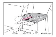
Slide the console box lid forward as needed. Pull the lid forward by holding the front of the lid.
