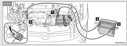
Connect the jumper cables according to the following procedure:
