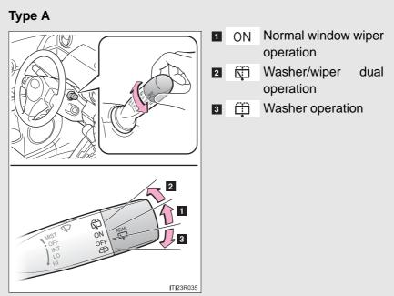
The wiper operation is selected by moving the lever as follows:
