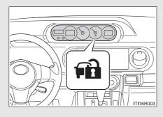
The indicator light flashes after the key has been removed from the engine switch to indicate that the system is operating.
