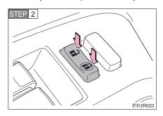
Shift the shift lever to P or N, and press and hold the driver's door
