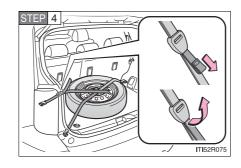
Make sure the flat tire is stowed securely by tightening the belt firmly using the adjuster.
