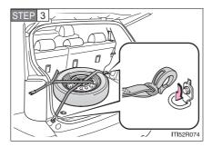
Hook another end of the belt (ivory portion) coming through the center hole to the other front cargo hook, and the other end (dark gray portion) to the rear cargo hook located diagonally to the secondly used front hook.
