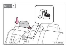
Secure the child restraint system using the seat belt or the LATCH anchors, and move the head restraint in place at the lowest position.
