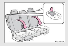
Fold the seatback down while pushing the seatback lock release button.
