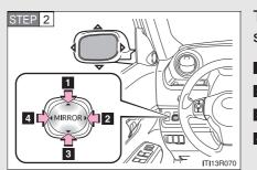
To adjust the mirror, press the switch.
