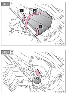
Disconnect the claws to remove the service cover as shown in the illustration.
