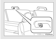
The coat hooks are provided with the rear assist grips.
