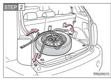
Put the flat tire on the center of the luggage mat with the outer side of the wheel facing up. Hook one end of the belt (dark gray portion) which is not forked to either front cargo hook.
