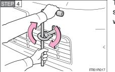
Tighten down the towing eyelet securely using a wheel nut wrench.
