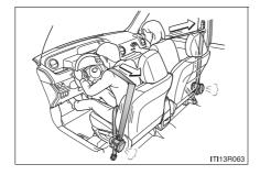
The pretensioners help the seat belt to quickly restrain the occupants by retracting the seat belts when the vehicle is subjected to certain types of severe frontal or side collision.
