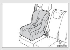
Seat belts equipped with a child restraint locking mechanism (ALR/ELR belts except driver's seat belt) (→P. 48)
