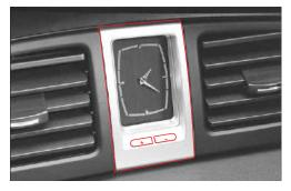
"+" button: minute pointer turns clockwise "-" button: minute pointer turns counterclockwise
