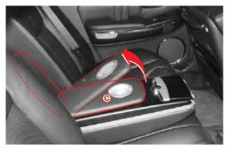
Pull up the center armrest's cover to open it. You can store small items in it (the power outlet and the AV jack are installed in the console box).
