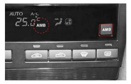
If you press the AMB switch, it will show you the ambient temperature for 5 seconds. It will be returned to its original display after displaying the temperature.
