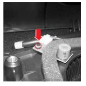
After replacing the filter, make sure to reset the timer to 0 by pressing the reset switch.
