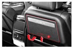
A table is on the rear of the passenger's seat for temporary jobs while the vehicle is stopping and putting on goods for rear seat occupants.
