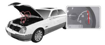
If the engine coolant temperature gauge indicates overheating or you have another reason to suspect that the engine may be overheating, stop and park the vehicle.
