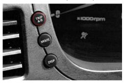
TRIP A/B switch is used for the display mode: TRIP A, TRIP B, and ODO (total driving distance)
