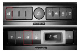
The rear fog light is activated when the tail lamp is on. The rear fog lights are located in the back-up lamp positions.
