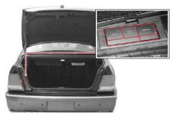
TV tuner and navigation system is installed on the upper part of the trunk. For more information, see separate multi-vision and navigation system manual.
