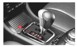
Select this position for normal forward driving on public roads and highways. At this position, the transmission is automatically shifted from the  $1\,\mathrm{st}$  gear through the  $5\,\mathrm{th}$  gear according to the vehicle speed.
