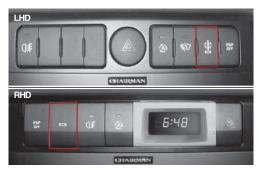
The electronical controlled ECS system minimizes the vertical vibration of the vehicle to enhance driving comforts and steering stability.
