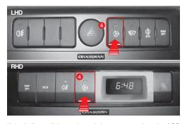
If the indicator light on the switch comes on when the AQS switch (4) is pressed, the AQS system is functioning properly.
