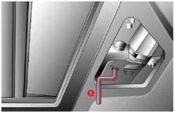
1. Manual operation hole and emergency crank
