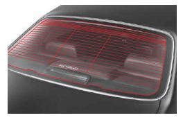
Glass antenna (for FM and AM) is on the upper and lower section of the rear window and the heating grids are on the center section of the rear window.
