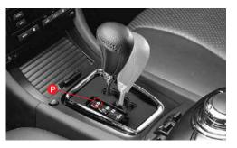
Select this position to park, start the engine, warm-up, and stop the vehicle for a long time.
