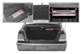
The changer is installed in the left bottom in the trunk and the navigation unit is installed in the trunk's upper side. For more information, refer to the navigation operating manual.
