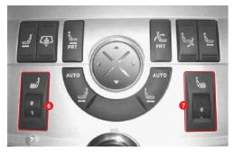
6: Rear Left Seat Heating Switch (control range: 1 to 5) 7: Rear Right Seat Heating Switch (control range: 1 to 5)
