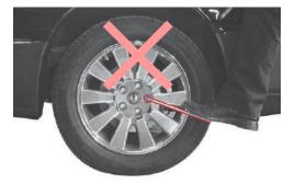
If over tightened, the wheel nuts could be damaged. Do not overtighten the wheel nuts by pressing the wheel nut wrench by foot or using an assist pipe.
