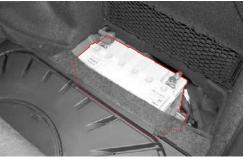
The MF battery is located at the right hand floor in trunk room. If the warning lamp in the instrument panel comes on while driving, turn off all electrical devices and have the system checked at the nearest Ssangyong Dealer or Ssangyong Authorized Workshop.
