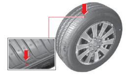
The tire tread wear indicators will appear when your tires have only 1.6mm of tread remaining (on the tire wall  $\blacktriangle$  indicator). When these indicators appear, replace your tires.
