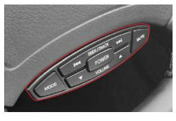
The remote audio control switch is located at the bottom of the steering wheel.
