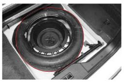
The temporary spare tire is only for an emergency. Do not use it for normal driving. The spare tire should be replaced with a regular tire as soon as possible.
