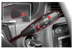
When the windshield wiper switch is at **AUTO** (1), the rain sensor (3) automatically turns on and off the wiper. And it controls the wiping speed by detecting the amount of rain drops.
