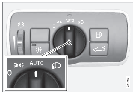
Headlight switch in the AUTO position
