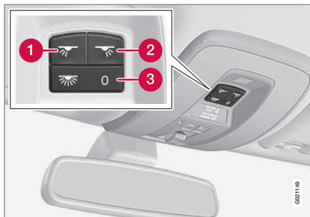
Light switches, front roof lighting
