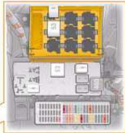
Relay carrier on left under dash panel
