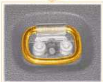
Lashing rings on floor
