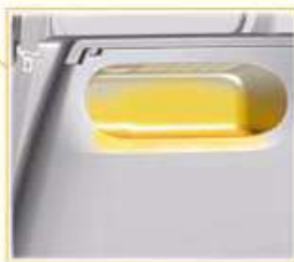
Storage between C and D-pillar
