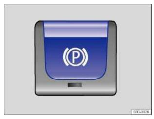
**Fig. 121** In the lower section of the center console: Electronic parking brake button.
