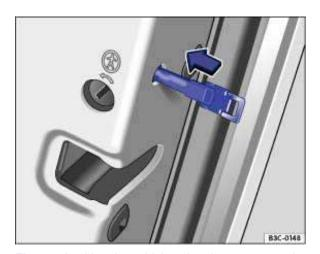
Fig. 163 Locking the vehicle using the emergency key.
