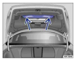
Fig. 26 Opened luggage compartment lid: Recessed grips for closing.
