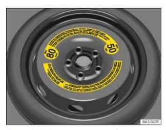
Fig. 156 In the luggage compartment: Compact spare wheel.
