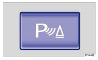
Fig. 126 In the center console: Button to switch the Park Distance Control system on or off.
