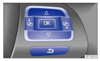
Fig. 12 Right side of the multi-function steering wheel: Controls for menus in the instrument cluster.
