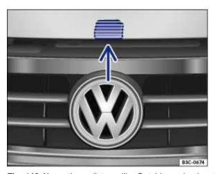
Fig. 142 Above the radiator grille: Outside engine hood release.
