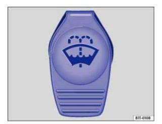
Fig. 83 In the engine compartment: Cap of the windshield washer fluid reservoir.
