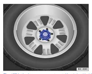
Fig. 155 In the luggage compartment: Handwheel holding spare wheel in place.
