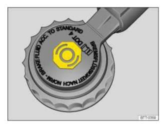
Fig. 123 In the engine compartment: Brake fluid reservoir cap.
