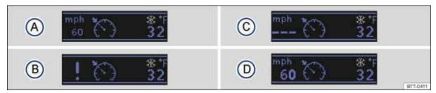
Fig. 132 In the instrument cluster display: Cruise control status indications.
