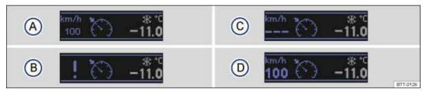
Fig. 133 In the instrument cluster display: Cruise control status indications.
