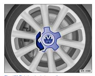
Fig. 172 Twisting the hubcap off.
