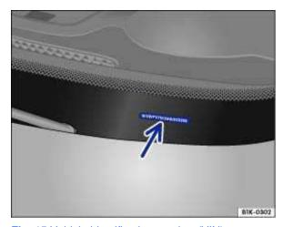
Fig. 15 Vehicle identification number (VIN).
