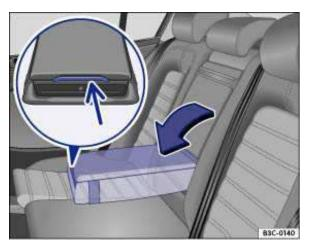
Fig. 104 Storage compartment in the rear center armrest.
