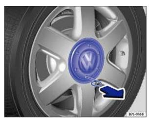
Fig. 171 Pulling the hubcap off.
