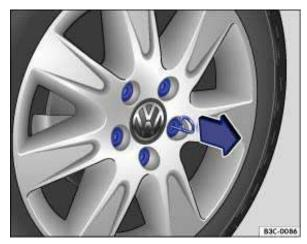
Fig. 174 Pulling cover caps off wheel bolts.
