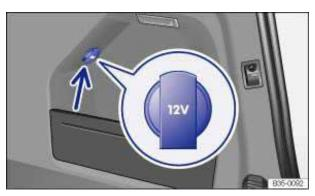
Fig. 110 In the luggage compartment: 12 Volt socket.
