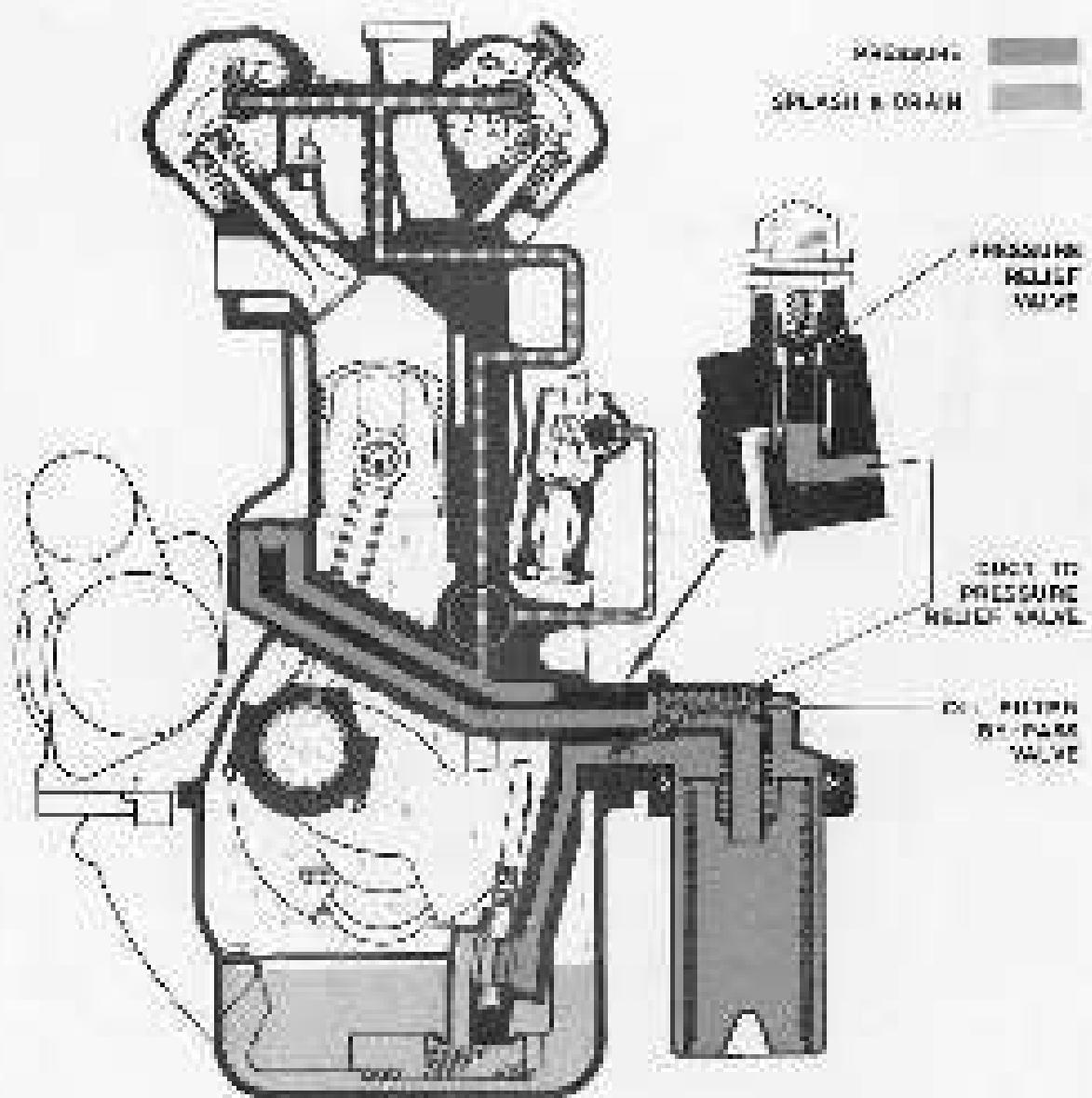
Fig. 5. Diagram of Type 15 and 16 Engine Lubrication system - front view.
