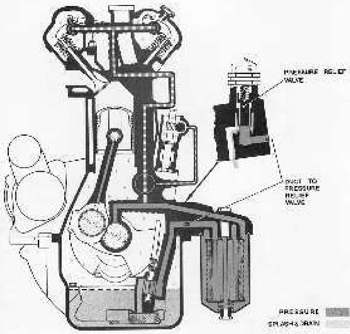
FIG. 2. Diagram of Type 177 Marine Lubricating Pump - front view.
