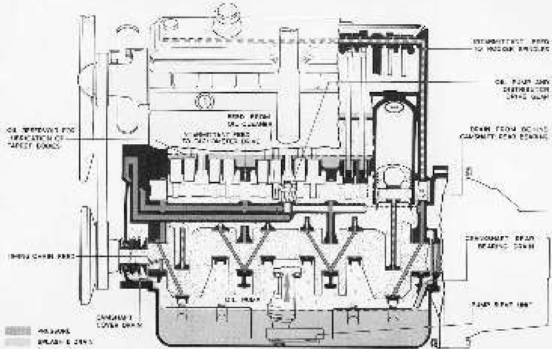
Fig. 3. Diagram of Type 85 and 86 Engine Lubrication System - Side View.
