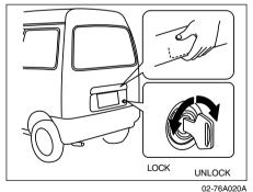
Lock or unlock the rearend door lock by inserting and turning the key. Turn the key left to lock and right to unlock the rearend door. Make sure the door is locked after locking by the key.
