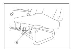
Fire extinguisher (1) is located below the rear seat as shown.
