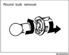
To remove a round bulb from a bulb holder, push in the bulb and turn it counterclockwise. To install a new bulb, push it in and turn it clockwise.
