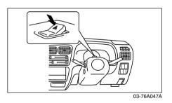
Push in the marked part of the hazard warning switch to activate the hazard warning lights. All four turn signal lights and both turn signal indicators will flash simultaneously. To turn off the lights, push the another side of the switch.
