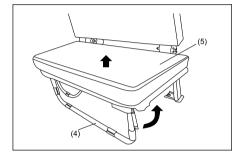
Fold rear seat leg (4) in direction as shown. Lift seat (5) up wards in order to fold it.
