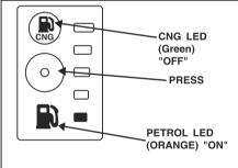
In this mode vehicle starts in petrol and continue running in petrol mode. In this mode, petrol indicator glows continuously in ORANGE color and CNG indicator (GREEN) will remain "OFF".
