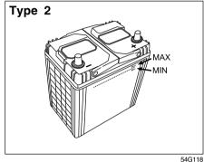
You should periodically check the battery, battery terminals, and battery hold-down bracket for corrosion. Remove corrosion using a stiff brush and ammonia mixed with water, or baking soda mixed with water. After removing corrosion, rinse with clean water.
