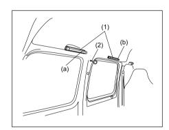
Tube lights (1) and hook (2) are located above the stretcher. Tube lights can be switched on by pressing switch (a) and (b) for individual tube lights.
