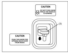
Back door can be opened from inside by pressing the knob downwards
