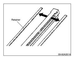
If the new blade is provided without the two metal retainers, move them from the old blade to the new one.
