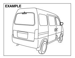
High mount stop lamp is provided on back door. The stop lamp will glow when the brake pedal will be depressed.
