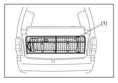
CNG cylinder (1) is installed in the luggage compartment, and is covered with protective cage (if equipped)
