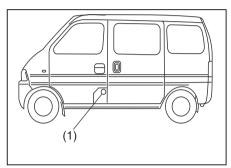
The CNG filler valve (1) is located on the left side of vehicle outboard.
