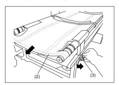
Pull pin (3) outwards in direction shown, in order to remove stretcher (2).
