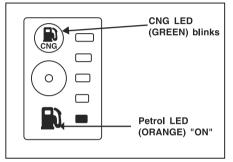
In this mode engine starts in petrol mode and then automatically changes to CNG after reaching programmed warming up condition. With ignition switch ON and vehicle started in "AUTO MODE", CNG indicator blinks (Green Color), and PETROL indicator glows (Orange color) continuously.
