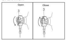
CNG supply can be switched off by closing the manual shutoff valve.
