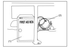
First aid box (1) and oxygen cylinder clamp (2) are located below stretcher.
