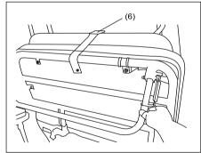
Using strap (6) fold the seat as shown in the figure.
