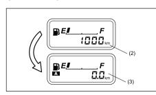
The odometer (2) records the total distance the vehicle has been driven. The trip meter (3) can be used to measure the distance travelled on short trips or between fuel stops.
