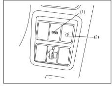
Switches for Siren and Revolving light are located on dash board on right side of steering wheel. Press Siren switch (1) for activating Siren and push again to deactivate. Press switch (2) for revolving light and push again for switching off.
