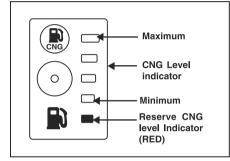
CNG level indicator is built into thechangeover switch. It consists of four green and one red LEDs, which indicates approximate amount / level of remaining CNG in the cylinder. Red LED of CNG level indicator glows when reaches to reserve quantity.
