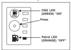
This is emergency mode and may be used in cases where there is no petrol in petrol tank. In this mode vehicle starts in CNG and continues running in CNG mode. With ignition "ON" and engine not running, press and hold the changeover switch till CNG indicator glows continuously. In this mode, CNG indicator glows continuously in GREEN color and Petrol indicator (ORANGE) remains "OFF".
