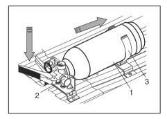
Insert the body of fire extinguisher (1) in to the clamp (3) and place the nozzle (2) carefully downwards, on the clamp
