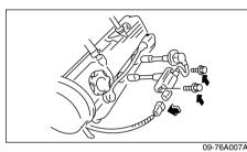
You should inspect spark plugs periodically for carbon deposits. When carbon accumulates on a spark plug, a strong spark may not be produced. Remove carbon deposits with a wire or pin and adjust the spark plug gap.
