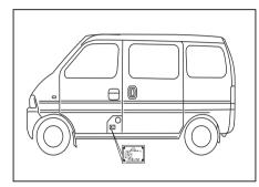
CNG cylinder identification number and CNG kit installation date is located below CNG filler valve as shown.
