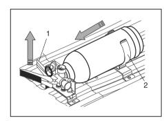
Lift Lever (1) of fire extinguisher slightly upwards and pull the fire extinguisher in the direction as shown in the figure, in order to disengage it from clamp (2).
