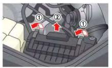
Remove the retainers ① as illustrated and pull out the filter element ②.
