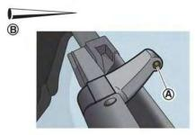
Be careful not to clog the washer nozzle (a). This may cause improper windshield washer operation. If the nozzle is clogged, remove any objects with a needle or small pin (B). Be careful not to damage the nozzle.
