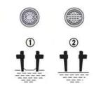
Check the fluid level in each cell (Remove the battery cover if it is necessary). It should be between the UPPER LEVEL ① and LOWER LEVEL ② lines.
