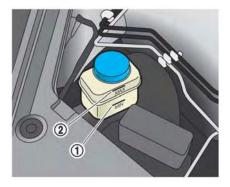
Check the fluid level in the reservoir. If the fluid is below the MIN line (1) or the brake warning light comes on, add Genuine NISSAN Brake Fluid R35 Special II fluid up to the MAX line (2). If fluid must be added frequently, the system should be checked by a GT-R certified NISSAN dealer.
