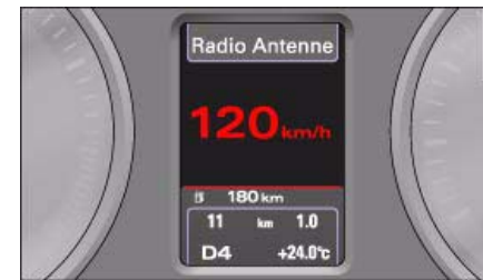
Fig. 13 Display: Digital speedometer
