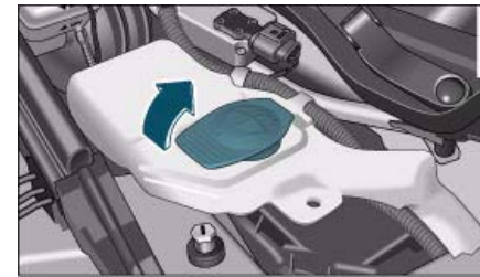
Fig. 230 Engine compartment: Windscreen washer container
