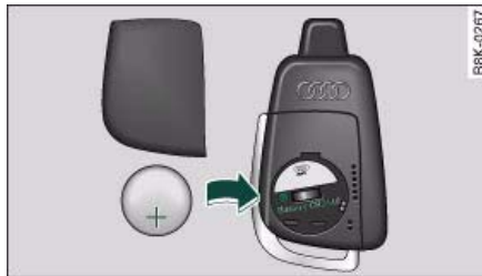
Fig. 131 Remote control: Changing battery
