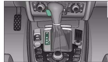
Fig. 144 Detail of the centre console: Selector lever with interlock button
