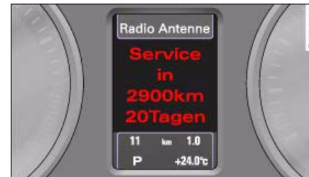
Fig. 16 Instrument cluster display: Service interval display
