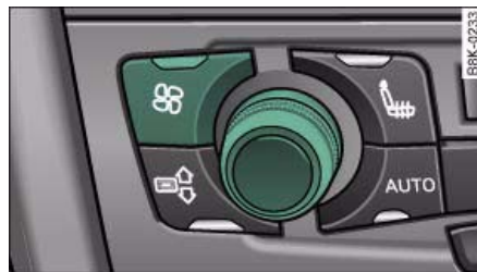
Fig. 119 Blower button and rotary control
