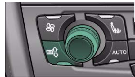
Fig. 121 Air distribution button and rotary control
