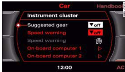
Fig. 12 MMI display: Switching the suggested gear on and off
