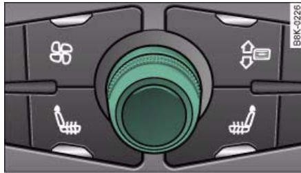
Fig. 107 Rotary control for temperature selection
