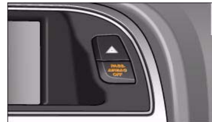
Fig. 196 Lamp indicates that front passenger's airbag has been deactivated via key-operated switch
