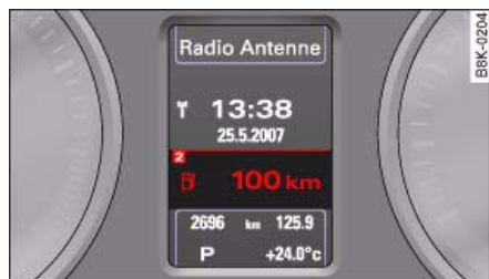
Fig. 17 On-board computer: Fuel range
