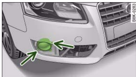
Fig. 270 Screws securing fog light
