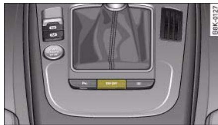
Fig. 203 Without MMI: Centre console with ESP switch
