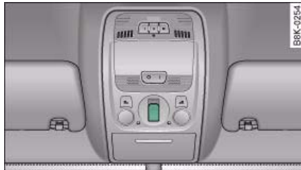
Fig. 47 Detail of headliner: Switch for tilting panorama roof
