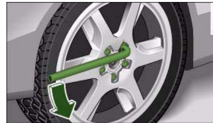
Fig. 242 Changing a wheel: Loosening wheel bolts
