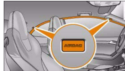
Fig. 193 Location of head-protection airbags above the doors
