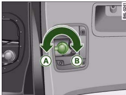
Fig. 257 Diagram: Bulb holder with a bayonet fastener
