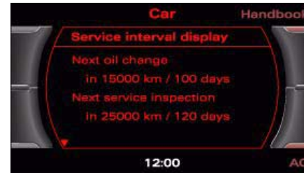
Fig. 15 MMI display: Service interval display
