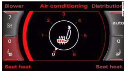
Fig. 132 MMI display: Seat heating
