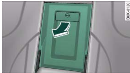
Fig. 92 In the rear seat: Opening the lid of the load-through hatch
