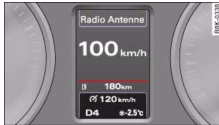
Fig. 141 Symbol and speed display while in cruise mode (short-term display)
