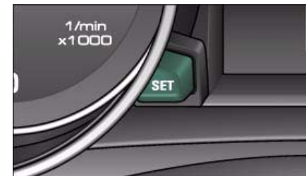
Fig. 22 Detail of the instrument cluster: SET button
