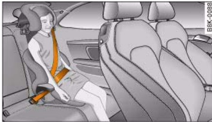
Fig. 199 A category 2/3 forward-facing child seat (with backrest) fitted on the rear seat
