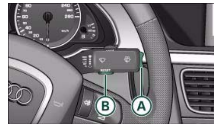
Fig. 20 Windscreen wiper lever: On-board computer controls
