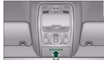
Fig. 105 Compartment for (sun)glasses in headliner
