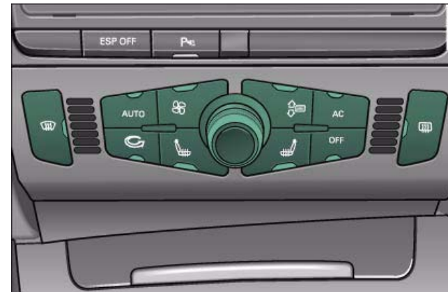
Fig. 106 Controls for deluxe automatic air conditioner
