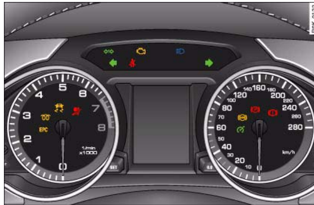
Fig. 7 Instrument cluster with warning and indicator lamps
