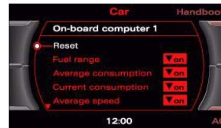
Fig. 21 MMI display: On-board computer
