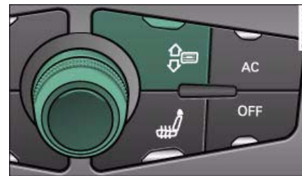
Fig. 111 Air distribution button and rotary control
