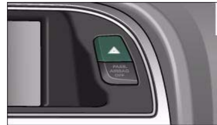
Fig. 56 Switch for hazard warning lights
