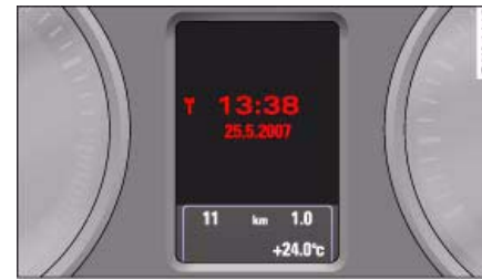
Fig. 4 Instrument cluster: Time and date display
