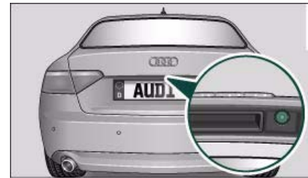
Fig. 154 Boot lid: Location of reversing camera
