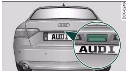
Fig. 43 Release catch on the boot lid
