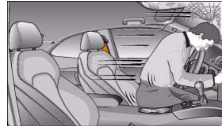
Fig. 180 A driver not wearing a seat belt can be thrown forwards
