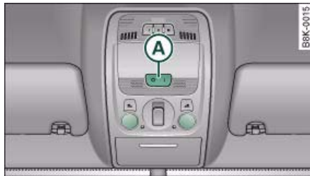
Fig. 58 Headliner: Front interior lights
