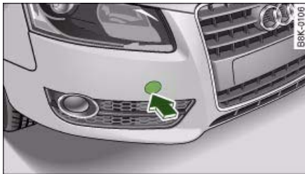
Fig. 250 Front bumper: Cover cap
