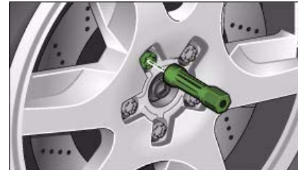
Fig. 245 Changing a wheel: Hexagonal socket in screwdriver handle to turn the wheel bolts after they have been loosened
