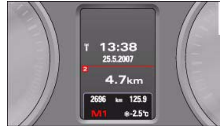
Fig. 148 Display: Manual gear selection (tiptronic mode)
