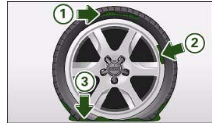
Fig. 239 The Tyre Mobility System is NOT suitable for repairing this type of damage to tyres.
