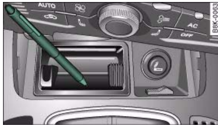
Fig. 151 Manual release of selector lever
