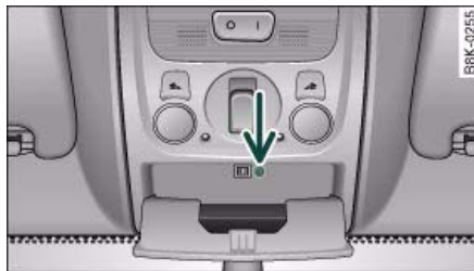
Fig. 48 Detail of headliner: Unscrewing the light housing
