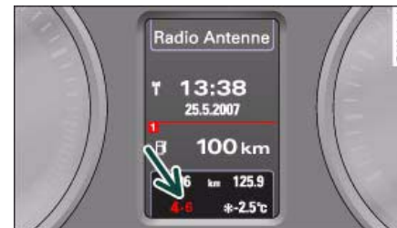
Fig. 11 Display: Gear-change indicator
