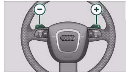
Fig. 149 Steering wheel: tiptronic switches
