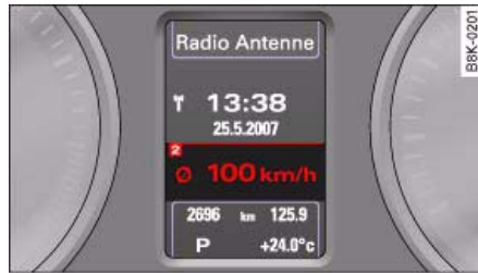
Fig. 8 Dashboard: Display in instrument cluster (automatic gearbox)
