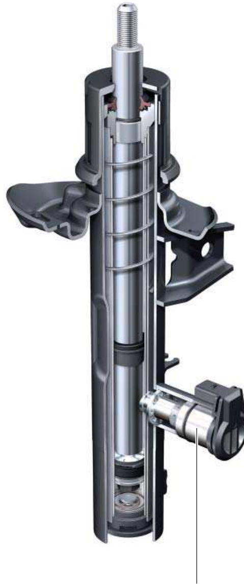
Electrically activated solenoid valve (damping adjustment valve)
