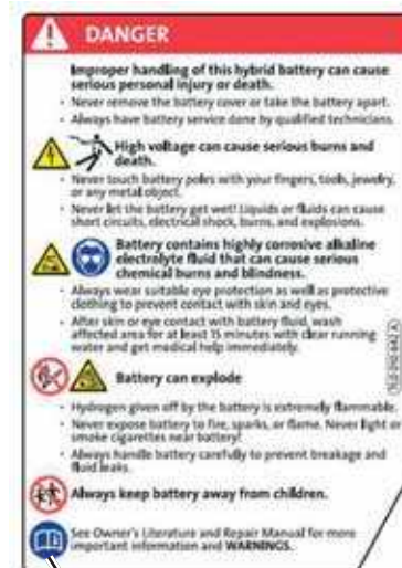
Special high voltage identification label affixed to the top of the battery in English and in the import country's national language
