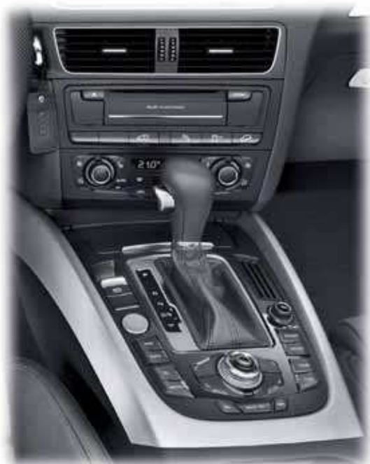
EV mode switch and shift control with tip-S function
