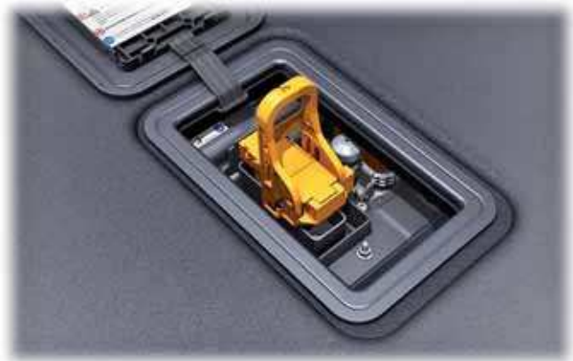
Maintenance connector in position 2
