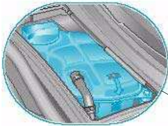
Coolant expansion tank
