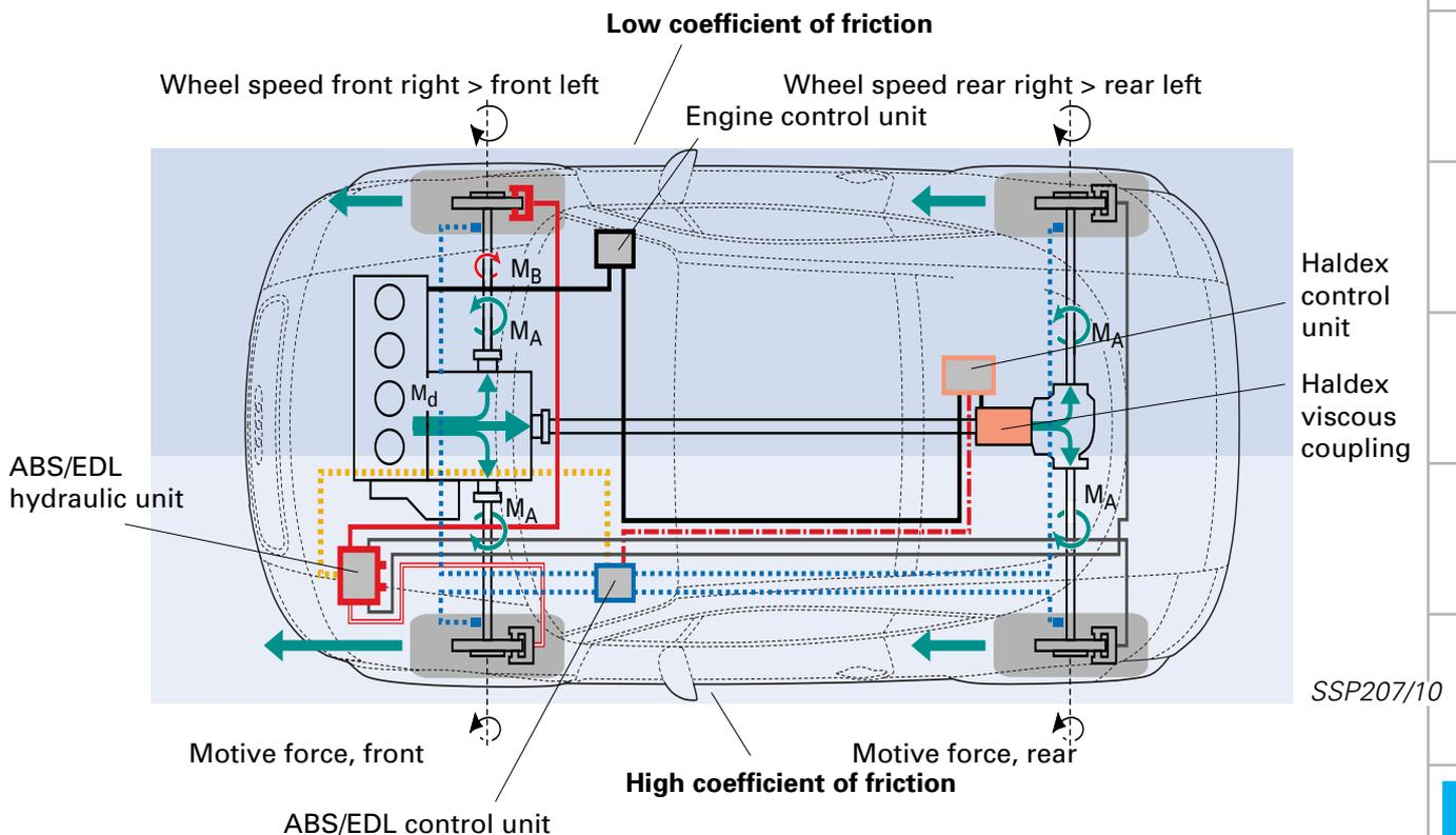
The Haldex viscous coupling does not have any sensors of its own apart from a temperature sensor (necessary for compensating for temperature-dependent oil viscosity).
