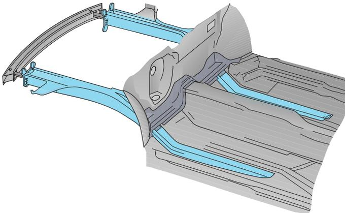
The vehicle front-end area deforms in a predefined manner, absorbing the impact energy without impairing the stability of the occupant cell. The side members are manufactured from 2-, 3- and 1.5-mm-thick mash-welded metal plates. In the case of a side impact, the strong cross members will also deform on the side of the body facing away from the impact to absorb some of the impact energy.
