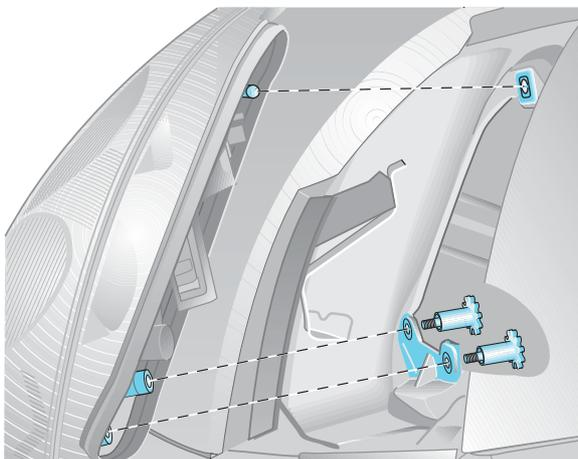
To replace the filament lamps, the complete taillight unit is removed without needing any tools. Flaps are attached to the luggage compartment linings on the left and right. The light cluster is secured on the inside by means of 2 captive knurled bolts. On the outside, the taillight is engaged in a ball head.
