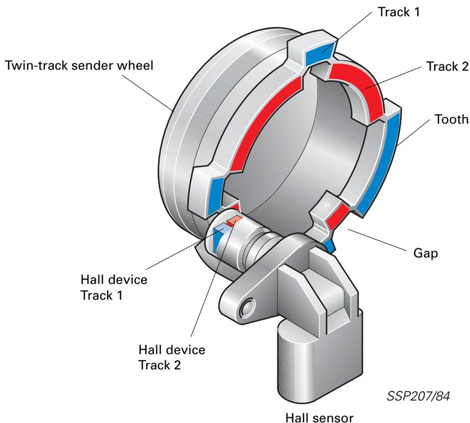
The quick-start sender wheel comprises a twin-track sender wheel and a Hall sensor. The sender wheel is designed so that two tracks are located side by side. In the position where there is a gap in one track, there is a tooth in the other track.
