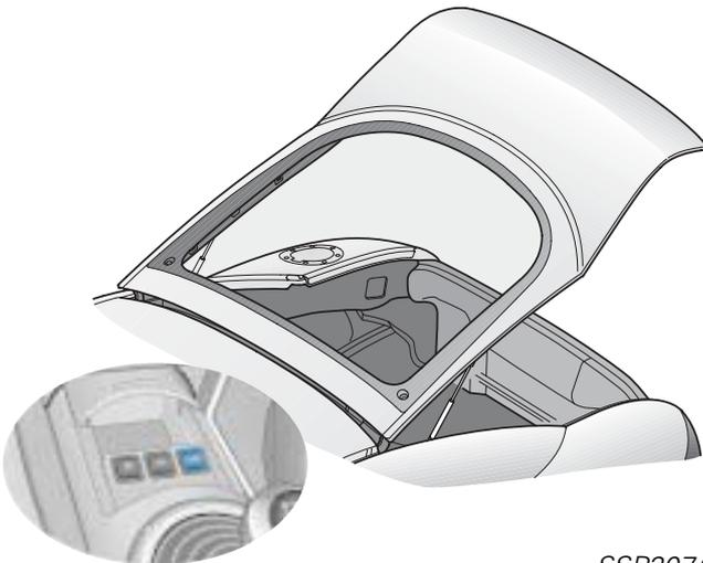
The tailgate can only be opened from the interior by means of the switch in the central console or by radio-wave remote control. The tailgate does not have a lock cylinder or a handle.
