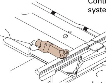
Lateral acceleration sensor, driver's side
