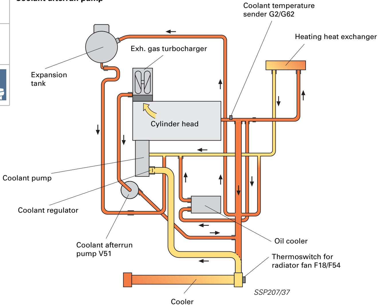
The exhaust gas turbocharger is water-cooled and integrated in the cooling circuit.
