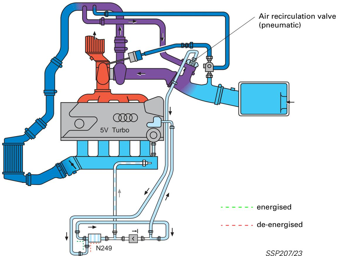
When the throttle valve is closed, it produces a backpressure in the compressor circuit due to the charge pressure still present. This causes the compressor wheel to decelerate rapidly. When the throttle valve is opened, the speed of the turbocharger must again be increased. The air divert control in overrun prevents turbo lag, which would otherwise occur.
