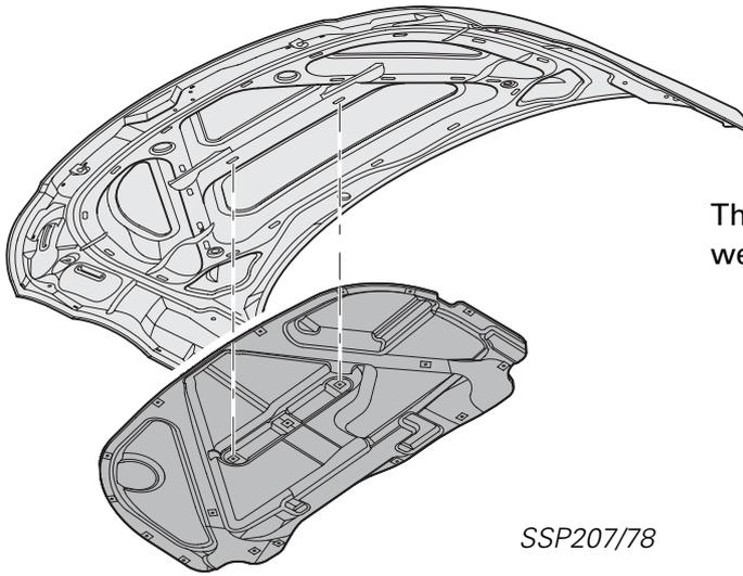
The bonnet is made of aluminium to save weight.
