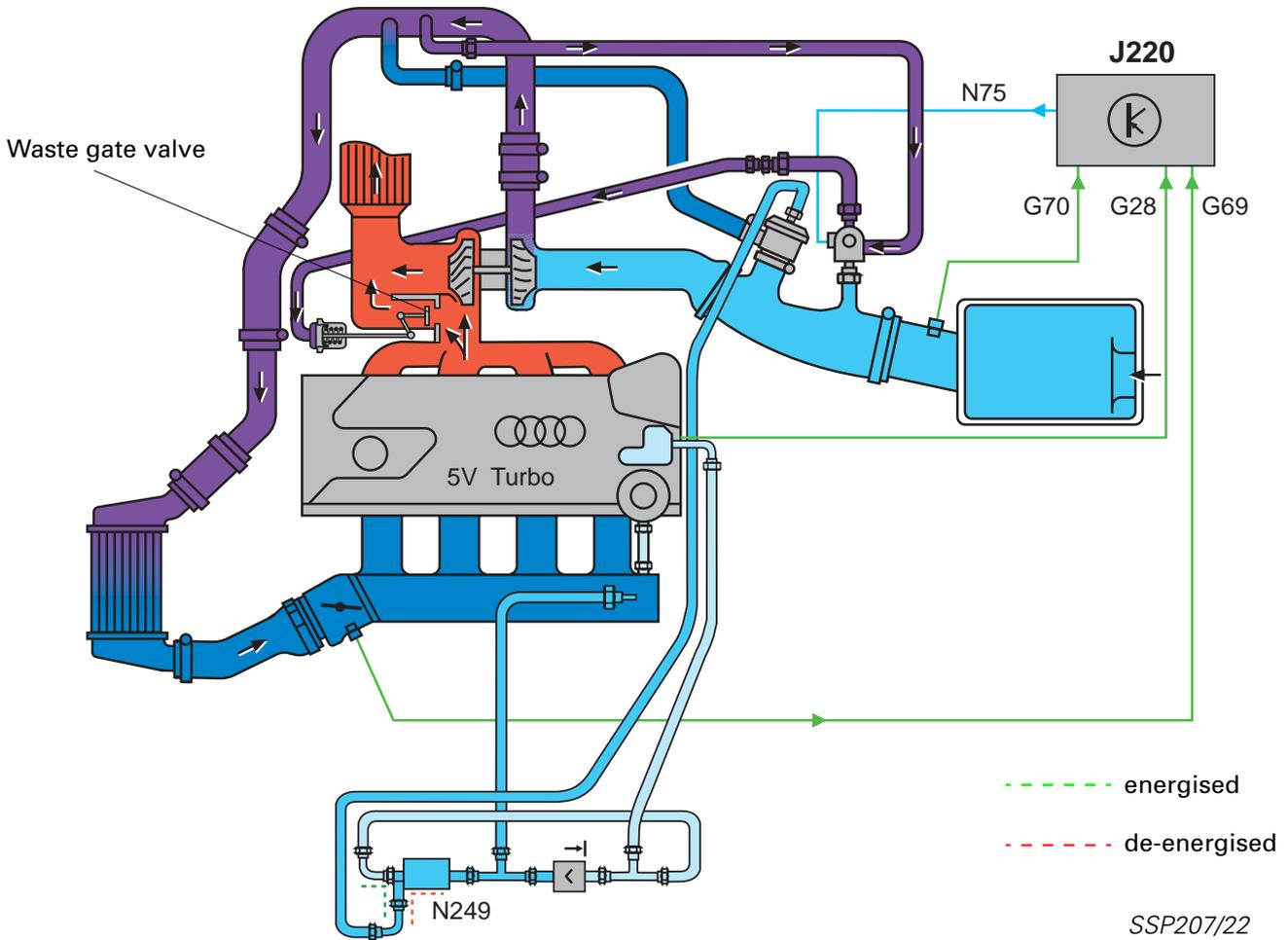
The engine control unit calculates the charge pressure setpoint from the engine torque request.
