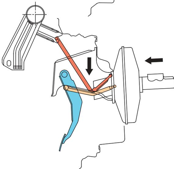
In the event of a frontal crash, the foot controls are displaced towards the central tube. This causes the collapsing support to deflect and the piston rod to buckle.
