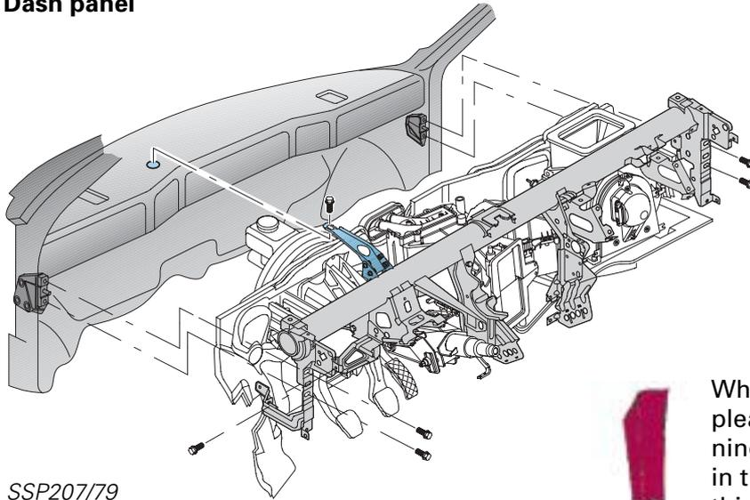
When removing the cross-tube, please note that one of the fastening bolts is located on the outside in the plenum chamber. To remove this bolt, it is necessary to remove the wiper linkage.
