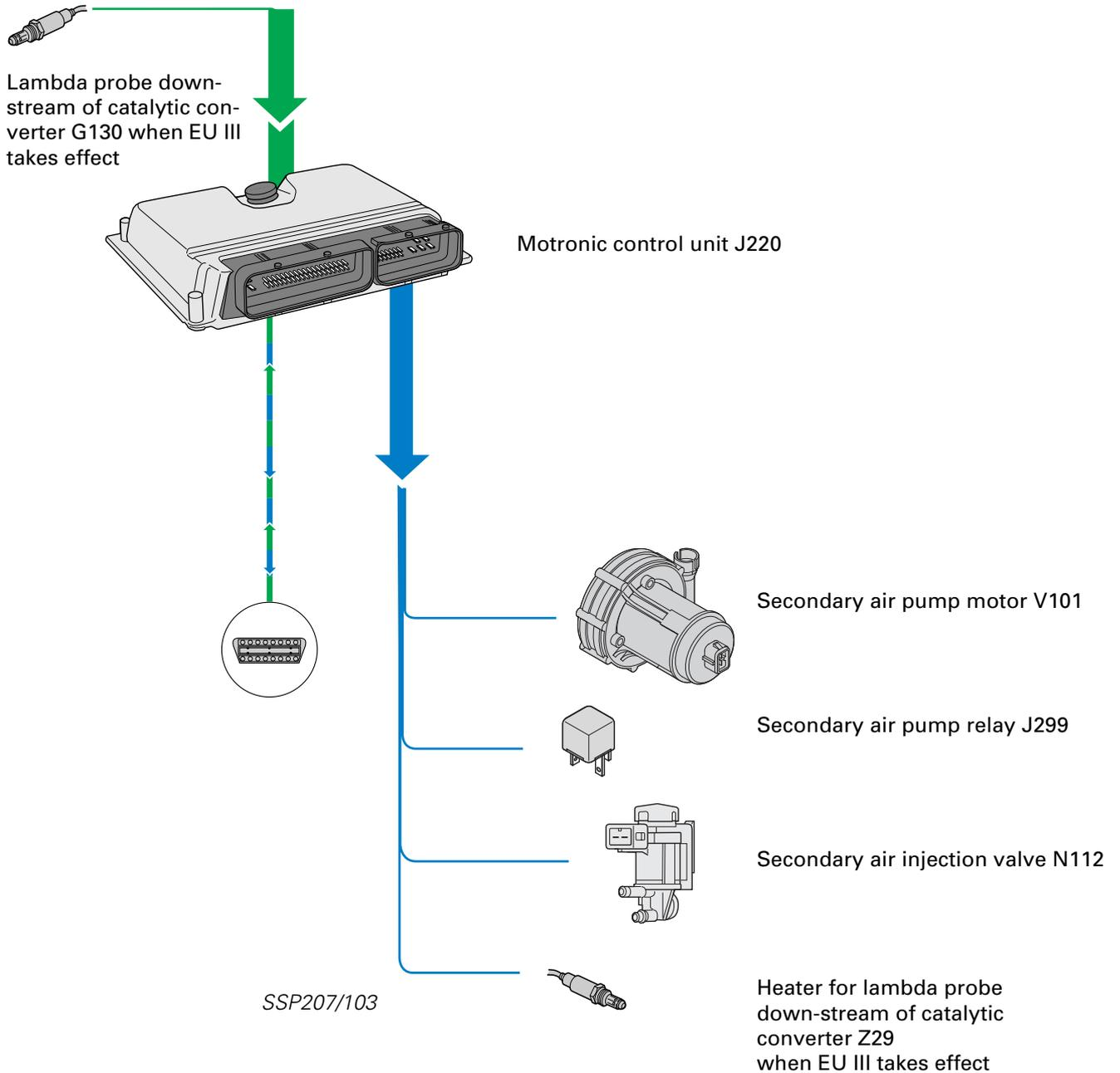
The secondary air system in the 1.8-ltr. 5V engine developing 165 kW ensures that the exhaust emissions comply with the EU III+D3 standard.
