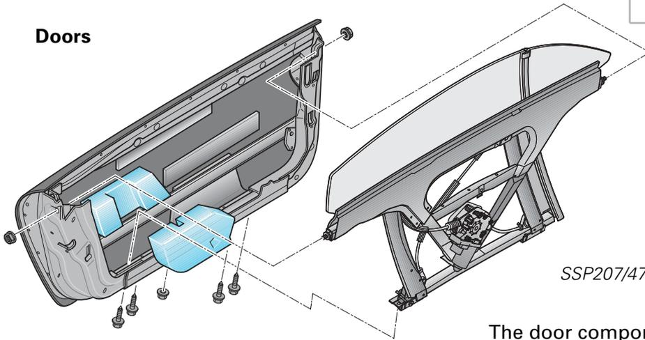
The doors of the Audi TT Coupé are frameless and of two-piece construction. The door panel is made of steel with a bolted high-strength side reinforcement integrated in the door.
