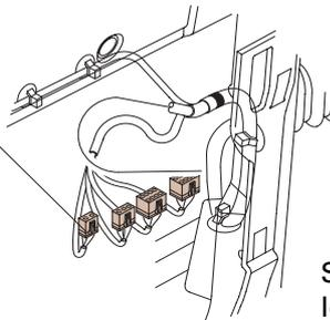
Socket (power windows, loudspeaker, radio, central locking, anti-theft alarm)
