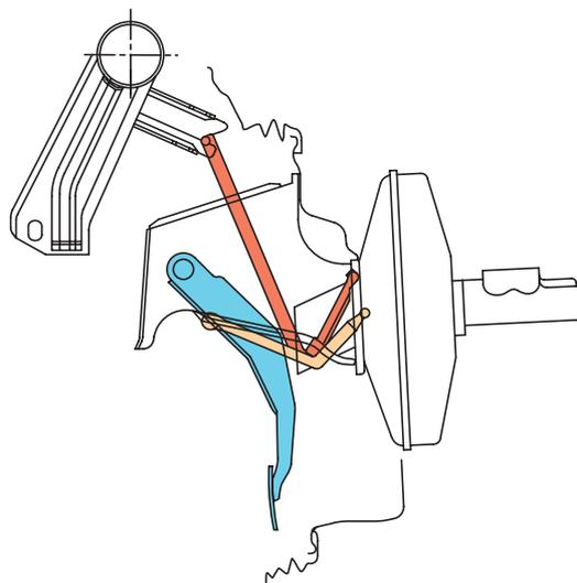
The pedal footplate is swung up to 170 mm away from the foot area.
