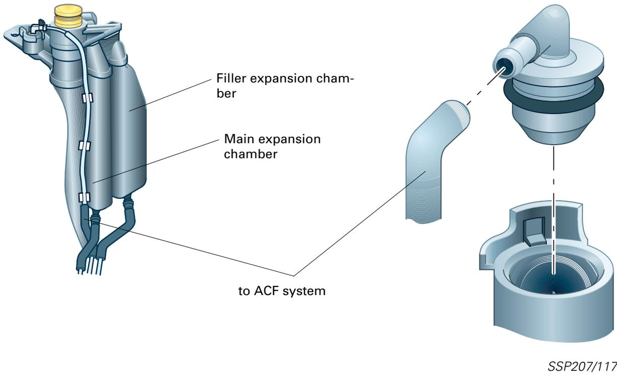
The gravity float valve prevents fuel from entering into the ACF system when cornering at high speed or if the vehicle rolls over.
