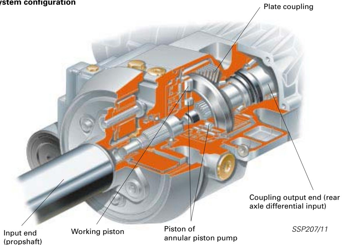
The Haldex viscous coupling is accommodated in a closed housing and mounted in front of the rear axle drive.
