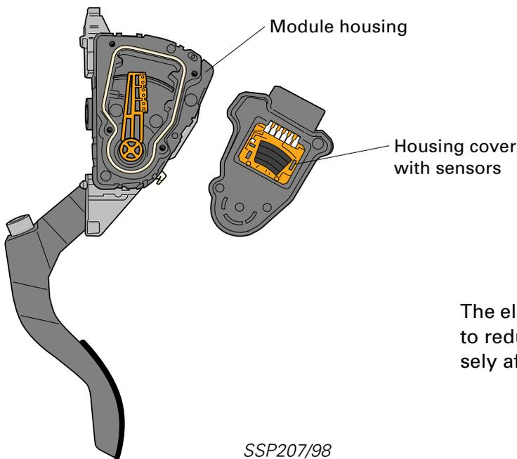
The electronic throttle control function is used to reduce and increase torque without adversely affecting the exhaust emission values.
