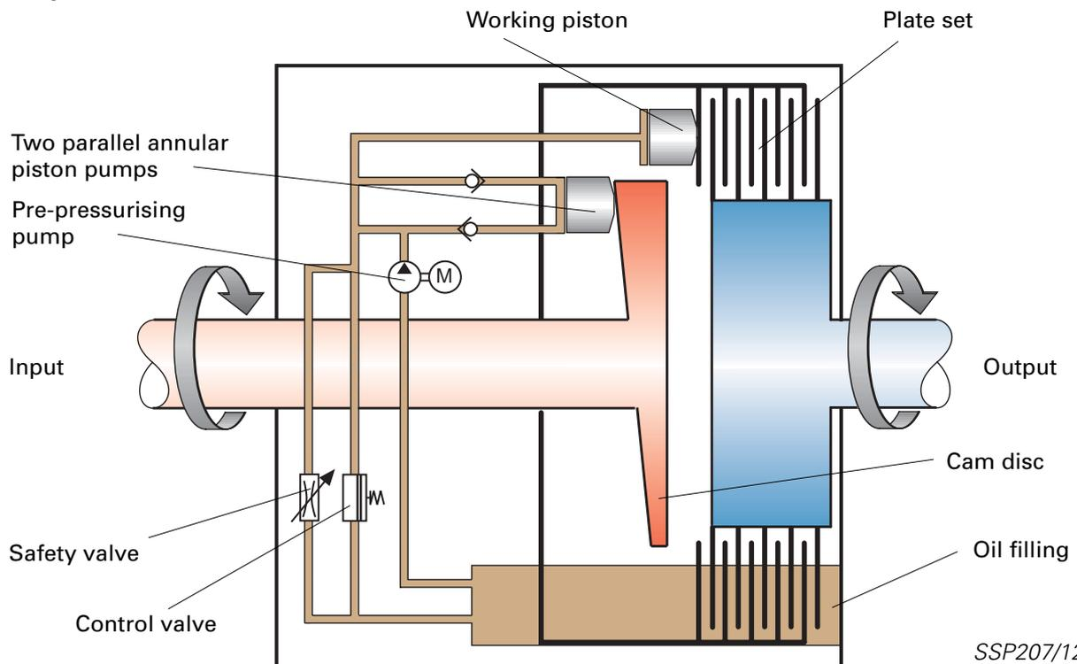
Torque is transmitted to the rear axle drive by means of the plate coupling .
