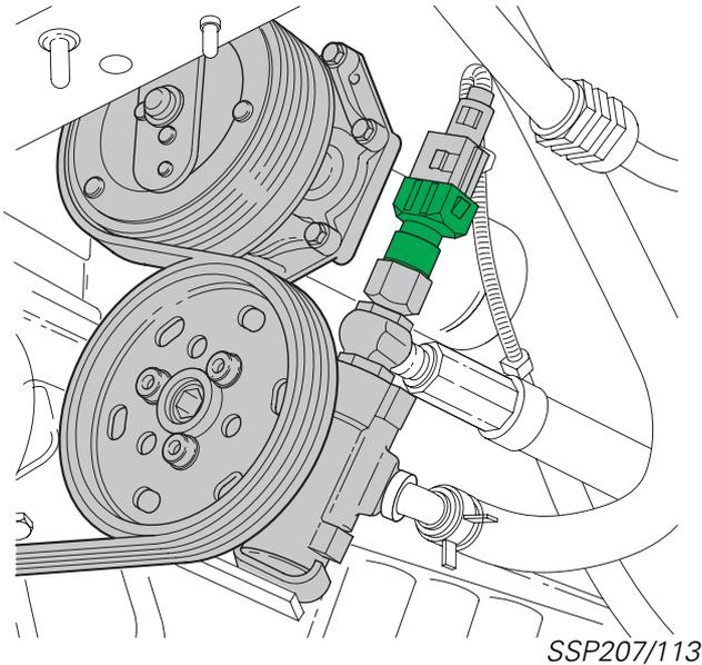
The pressure switch for power steering is located on the vane pump. It informs the engine control unit when the vane pump is subjected to a load.
