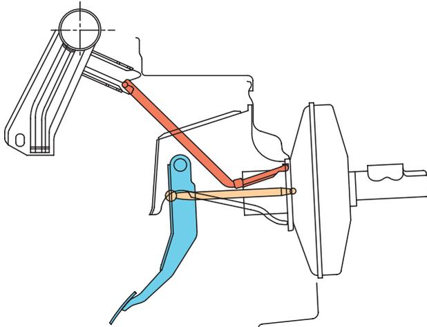
To minimise the risk of foot injuries in serious head-on collisions, the brake pedal is swung away from the foot area by means of a collapsing support if severe deformation of the vehicle occurs.
