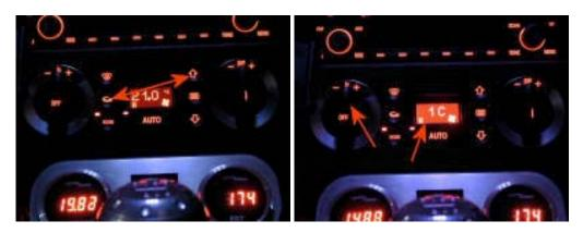
Twist the temperature dial to cycle trough the codes. Then press the recirculation button again to enter the code. The value should display:
