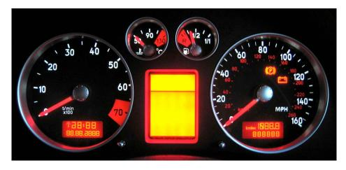
5. **Illumination test.** The illumination switches to dark, brightens, then dims down again, and finally switches back to the original brightness.
