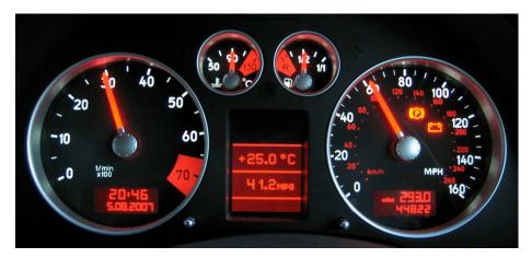
2. Warning lamp test. Lamps are lid (not all, though).
