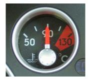
The fuel and temp gauge readings can be also checked against the fuel level and the coolant temperature values in VAG-COM. To enter the measuring block, select *Instruments*, then hit *Meas. Blocks – 08:*
