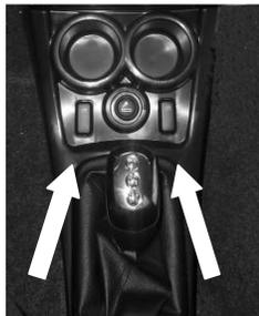
The two electric window control switches are located at the bottom of the dashboard's central facade.
