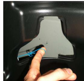
Pull the safety handle (blue cable) in order to unlock the tailgate chest.
