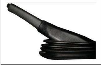
1. To put on the brake, completely pull the lever without pressing the button at the end of the lever.
