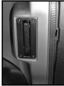
Pull the handle located under the safety belt on the left inner panel. Raise the tailgate to its maximum position without forcing, the two jacks will hold it open.
